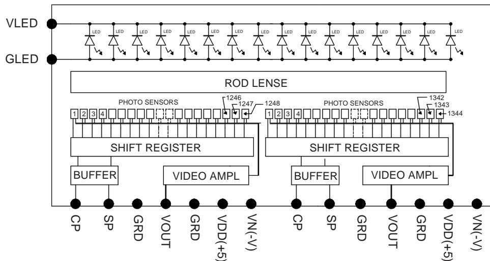
Figure 1. PI324MC-A4 module block diagram.
